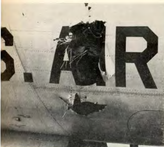
Damage to aircraft is shown in these photos. Shell bursts caused loss of hydraulic fluid, put electrical systems out of commission, and injured navigator.
